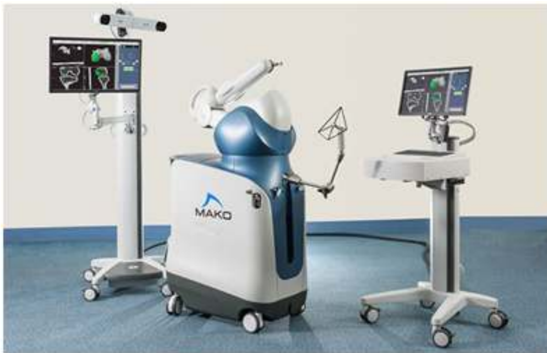
Fig. 4 : MAKO Robot for Knee Replacement
